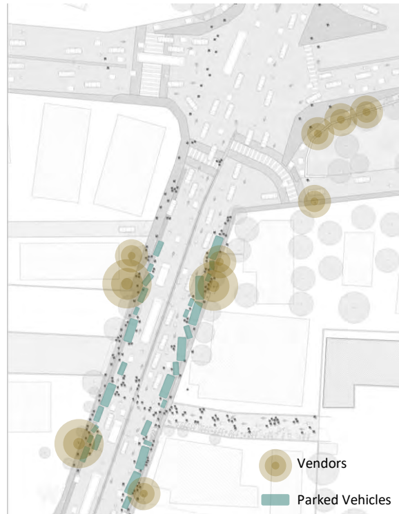
Vendor and parking encroachments force children to walk on the carriageway.
