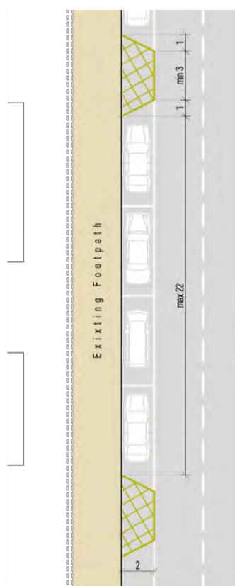
Typical bay with parking slots for cars
